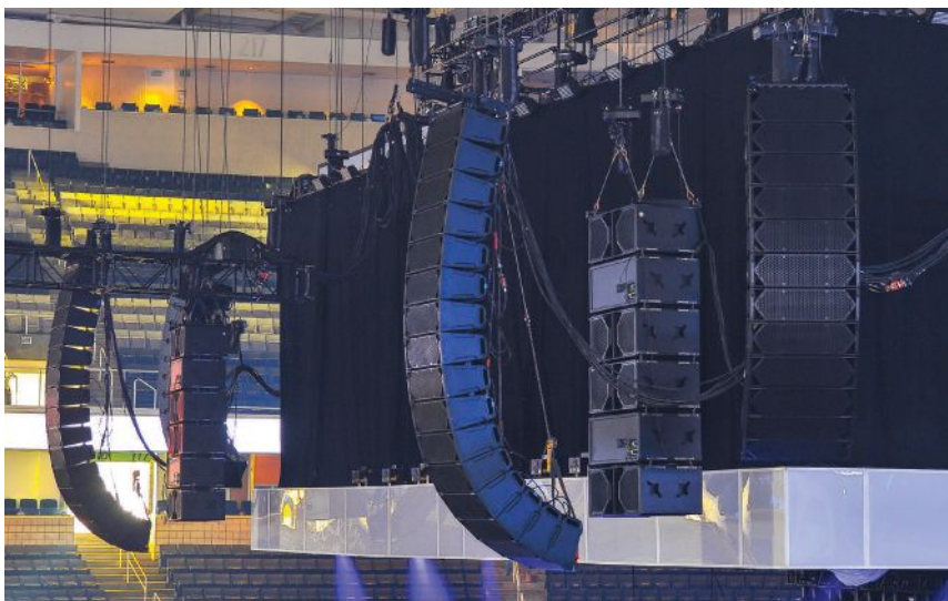
The main PA arrays comprised of Clair Global Cohesion CO-12 arrays and CP-218 subwoofers.
