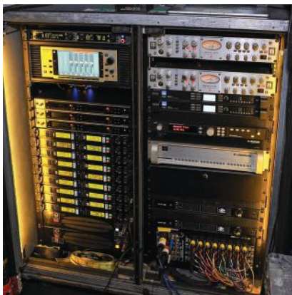
Morales' effects rack joined by the tour's Shure PSM 1000 wireless transmitters for monitoring and Sennheiser Digital 9000 wireless mic receivers.
